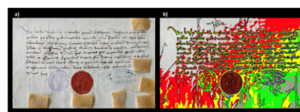
left: EVA strips applied to one of the letters. right: Fluorescence measurement of phenylalanine, tyrosine & tryptophan
