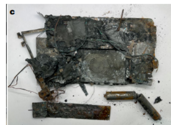
Remains of the laptop causing the fire.
